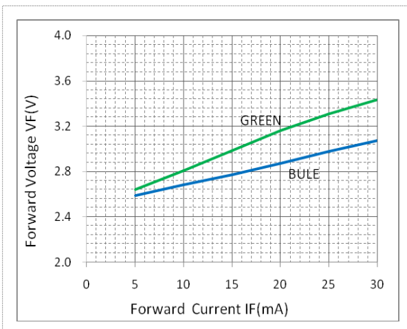
Fig 5. Forward Current vs. Forward Voltage, Ta=25°C
